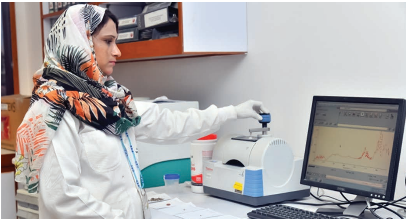
Technologist performing renal stone analysis of a pediatric renal stone using Fourier Transform Infrared Spectroscopy. The most common component reported in pediatric age group is ammonium hydrate.
