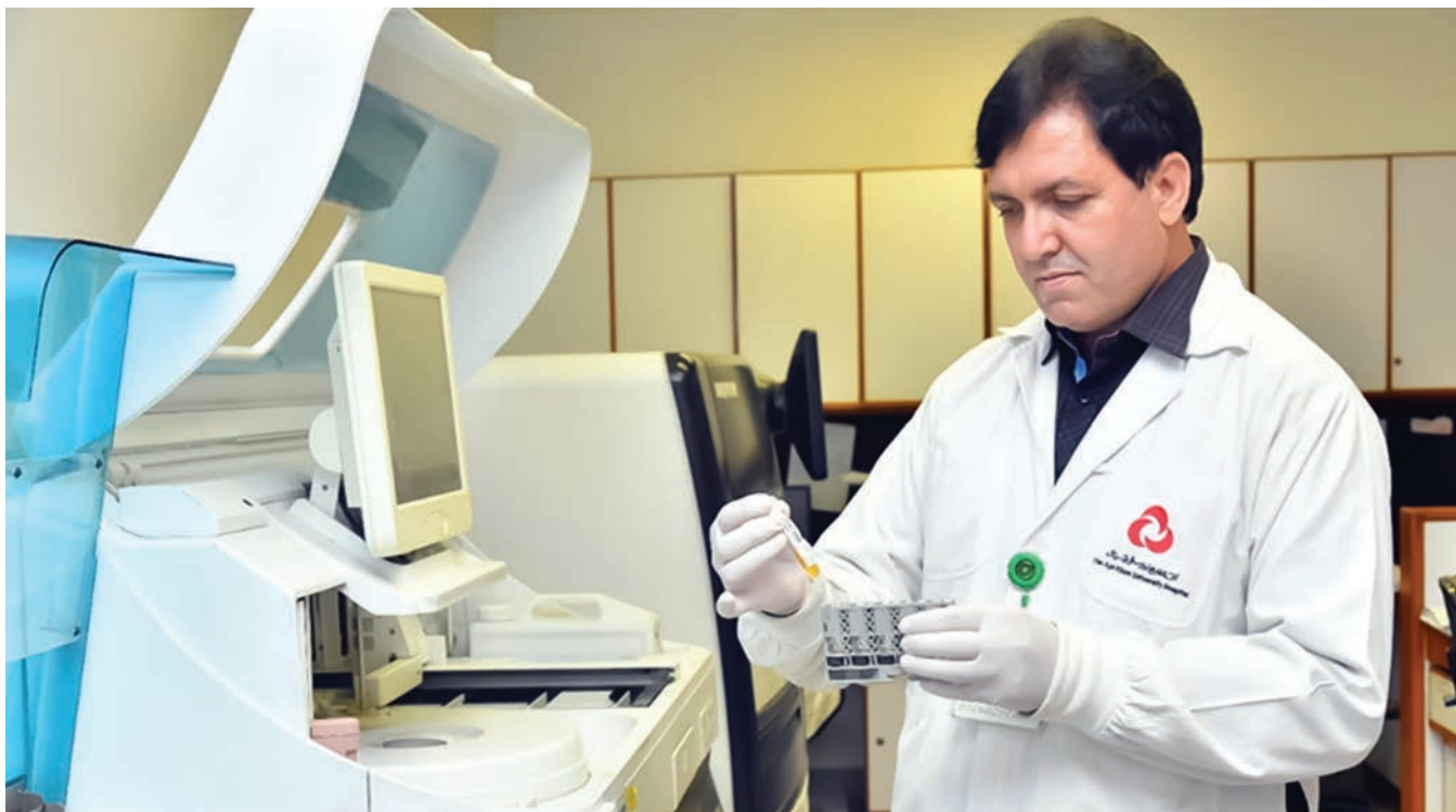
Technologist performing the Thyroid Receptor antibodies (TRAb) using Electrochemiluminescence Immunoassay methodology on the Cobas e411 analyzer (Roche Diagnostics, US)
