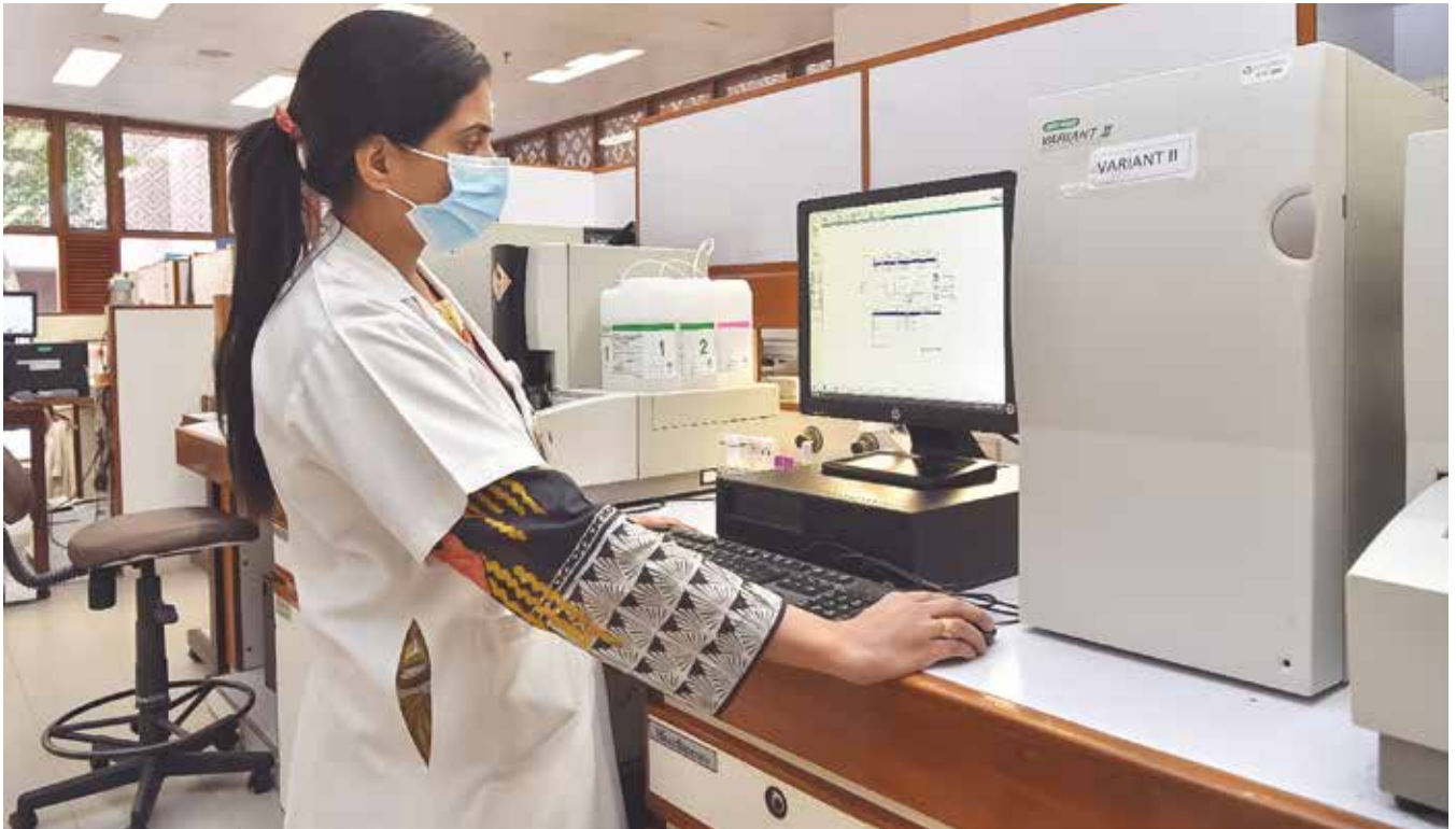
Picture 3: Haematology resident analyzing hemoglobin variant chromatograph generated by high performance liquid
