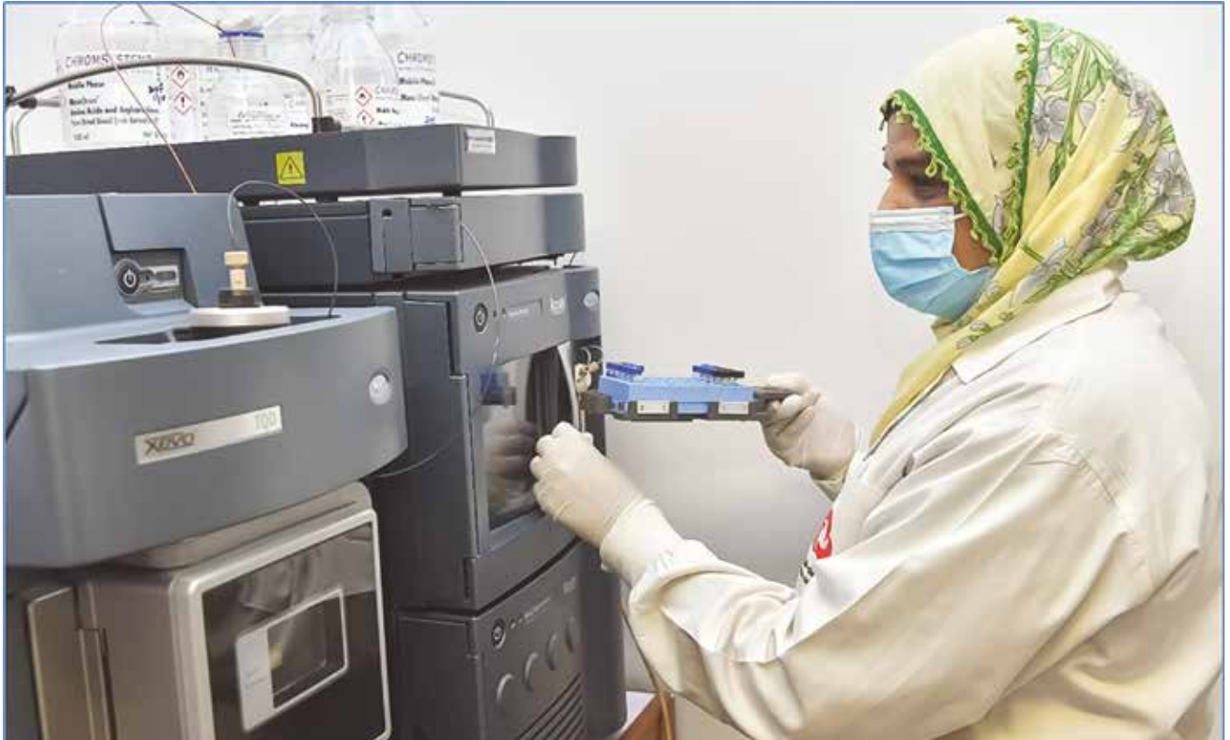
Picture 7: Technologist analyzing dried blood spot specimen for Acylcarnitine on Liquid Chromatography-Mass Spectrometry
