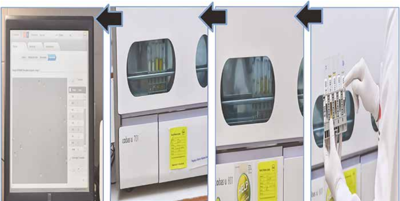
Picture 1: Integration of urine chemical and microscopic analysis. System perform picture analysis by neural network-based algorithm
